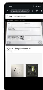
Scanning a device certificate from the Secure Card using a smartphone
