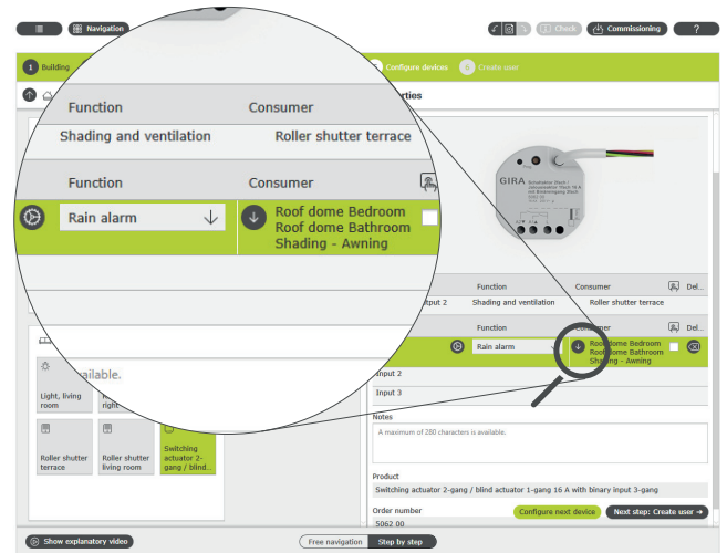
Assigning several devices to the "Rain alarm" function
