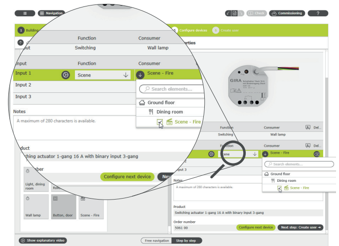
Assigning the "Fire" scene to the binary input
