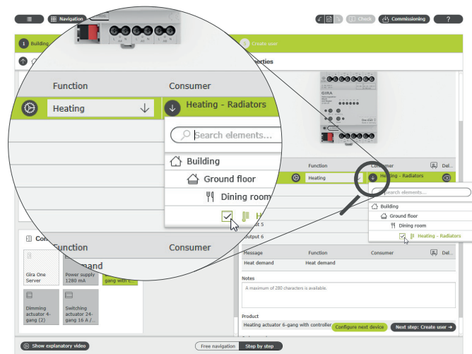
Choosing the “Heating” function and assigning devices
