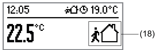
Figure 52: Example of a 2-area display with room temperature in the menu area and a large operating mode icon
