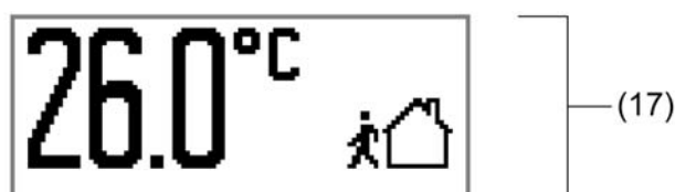
Figure 51: Example of a basic display with one display area (Room temperature, operating mode display)
