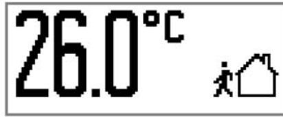
Figure 7: Example of a basic display with one display area (Room temperature, operating mode display)
