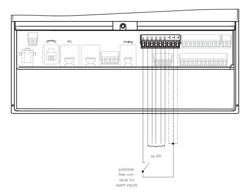
Between the connecting terminals M1 and **L** (mass potential) the desired switching contact is being connected. The voltage of the alarm input M1 in idle mode is 3.3 V. If the input is configurated as make contact, the desired action will be performed by the TeleCoppler 2 when making the contact. If the input is configurated as break contact, the desired action will be performed by the TeleCoppler 2 when breaking the contact.
