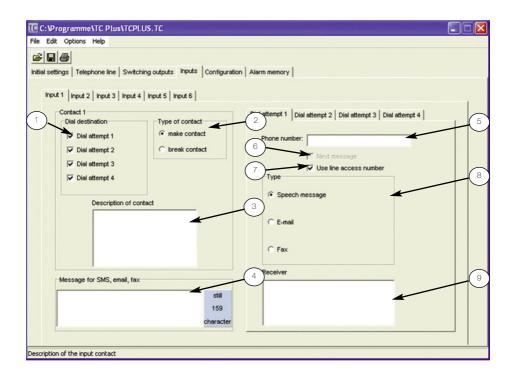
For the alarm inputs and the EIB inputs you can define the contacts. And to each contact you can define 4 destinations to which alarms should be sent. You can also define the type of message.
