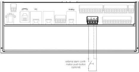
Using the external alarm confirmation push-button you can locally reset the alarm, i. e.
