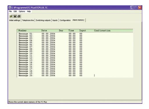
The last 20 messages will be saved in the alarm memory. These messages indicate date, time, alarm input and type of confirmation.
