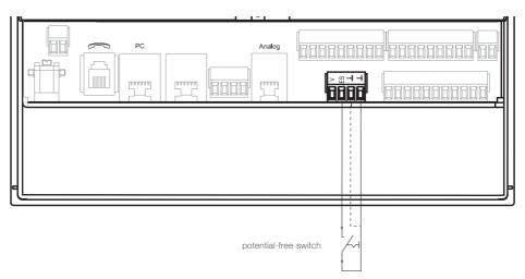
By closing an external potential-free switch the TeleCoppler 2 is switched transparent, i. e. without function. It has neither the function of re-
