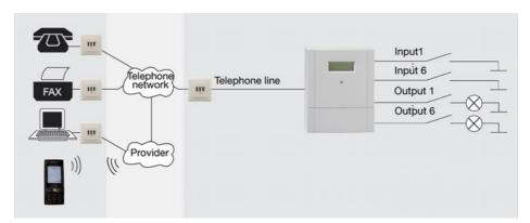
The above scheme shows the use of the TeleCoppler 2 with the analog telephone network. Alarm messages are transmitted via telephone line to the telephone network and from
