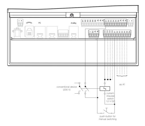
The TeleCoppler 2 is drafted for switching electrical devices by telephone. Each switching process by telephone is saved in the TeleCoppler 2. And on request, the announcement is made, whether the connected devices are switched on or off.
