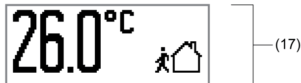
Figure 51: Example of a basic display with one display area (Room temperature, operating mode display)
