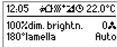
Figure 56: Example of a 2-area display with 2-line value display incl. supplementary text. Line 1 brightness value, line 2 slat angle
