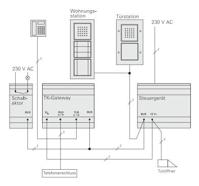
The single-family house has a door station, a home station with an additional call button, a switching actuator, which is to switch the outside light, and a TC-gateway. The TC-gateway is connected to the analogue telephone connection.
