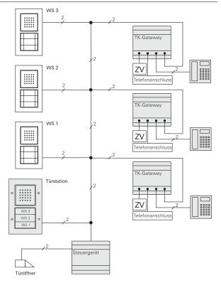
The house divided into several flats has a door station with three call buttons. There is a home station and a TC-gateway with an additional power supply (AS) in each of the flats.
