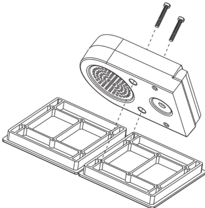
Use only the screws provided to mount the built-in loudspeaker.
