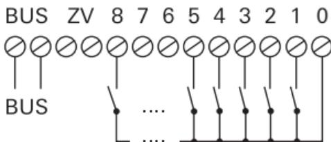
3. Connect the bell buttons. The maximum cable length is 2 m.
