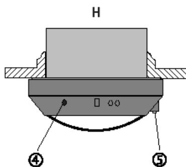
The presence detector standard attachment is then adjusted to the actual brightness prevailing at the monitored surface.
