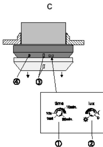
① Shut-off delay: 1 second (test operation).
