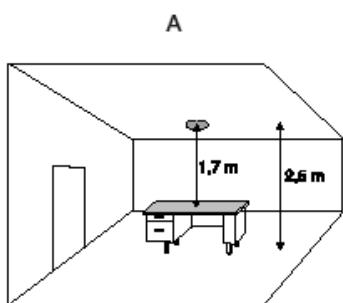
The detector works with a passive infrared sensor (PIR sensor) and responds to thermal movement triggered by persons, animals or objects. When movements are detected below a presettable brightness threshold, the detector switches on an electrical consumer. The device remains on as long as movements are detected.
