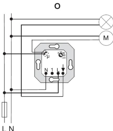
Connection of extension unit insert for presence detectors ① to main unit ② (e.g. Tronic switching insert) (figure Q).
