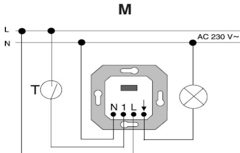
Combination of presence detector standard attachment with Tronic switching insert (figure **N**).
