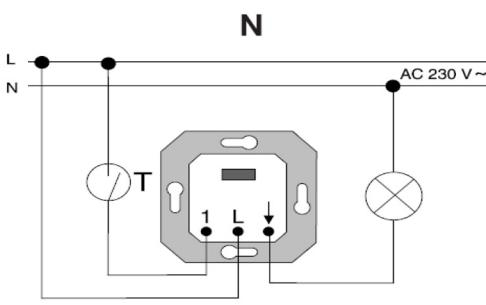
Combination of presence detector standard attachment with a HLK relay insert (fig. O).
