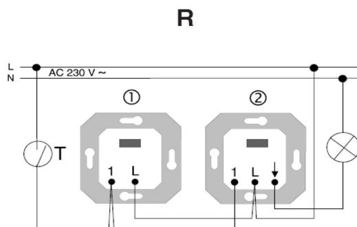
**When controlling the presence detector standard attachment through extension input 1 of the insert, please observe the instructions set out in the chapter "Use of extension units".**
