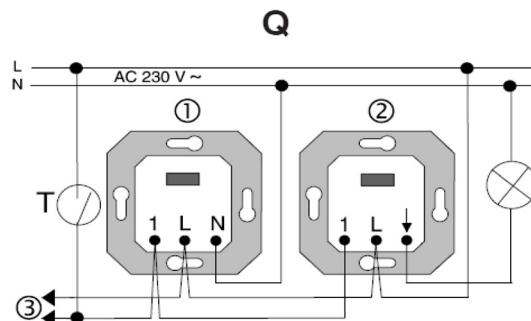
Combination of presence detector standard attachment with a 1-10 V control unit (fig. P)
