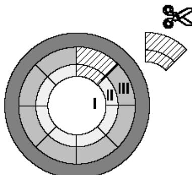
Cutting out the mask changes the diameter of the detection field on the floor as follows:
